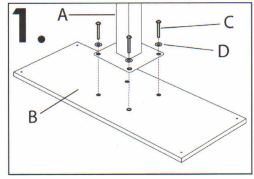
Align the Orbis Post (A) with one of the Ecoboard Panels(B). Pass the Socket Button Screws(C), with Washers(D), through the holes.
