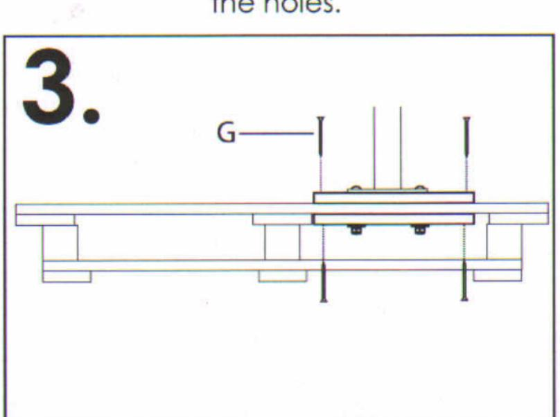
Secure the Ecoboard panels to the Pallet using the Woodscrews(**G**), through the predrilled pilot holes.
