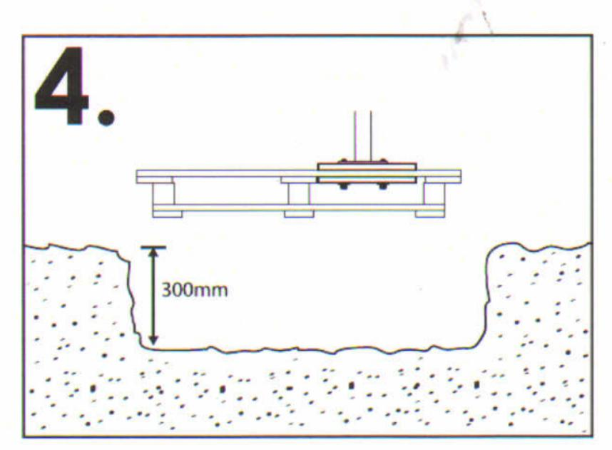
Excavate a 300mm deep hole in the sand to seat the bottom of the pallet. Ensure the bottom surface is level. Lower the full post assembly into position.
