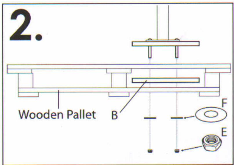
Sandwich the Pallet between the previous assembly, and the second Ecoboard (B) panel, and secure using M10 Nuts (E) with Plain Washers(F).
